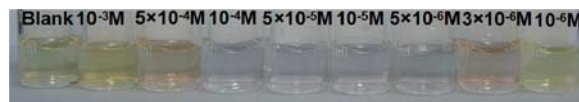
Fig. 10. Colorimetric visualization of BZKB using citrate-capped Ag NPs. BZKB concentrations varied from 10^{-6} M to 10^{-3} M.
